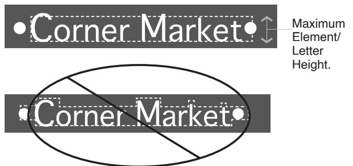
Figure 5-2: Measuring Wall Signs
